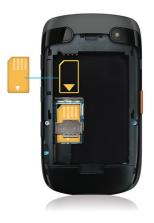
Slide the SIM card into the slot.
