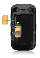
Slide the SIM card into the slot.
