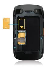
Slide the SIM card into the slot.
